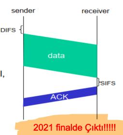
Recall that under Ethernet's CSMA/CD, multiple access protocol (Section 5.3.2), a station begins transmitting as soon as the channel is sensed idle. With CSMA/CA, however, the station refrains from transmitting while counting down, even when it senses the channel to be idle.
